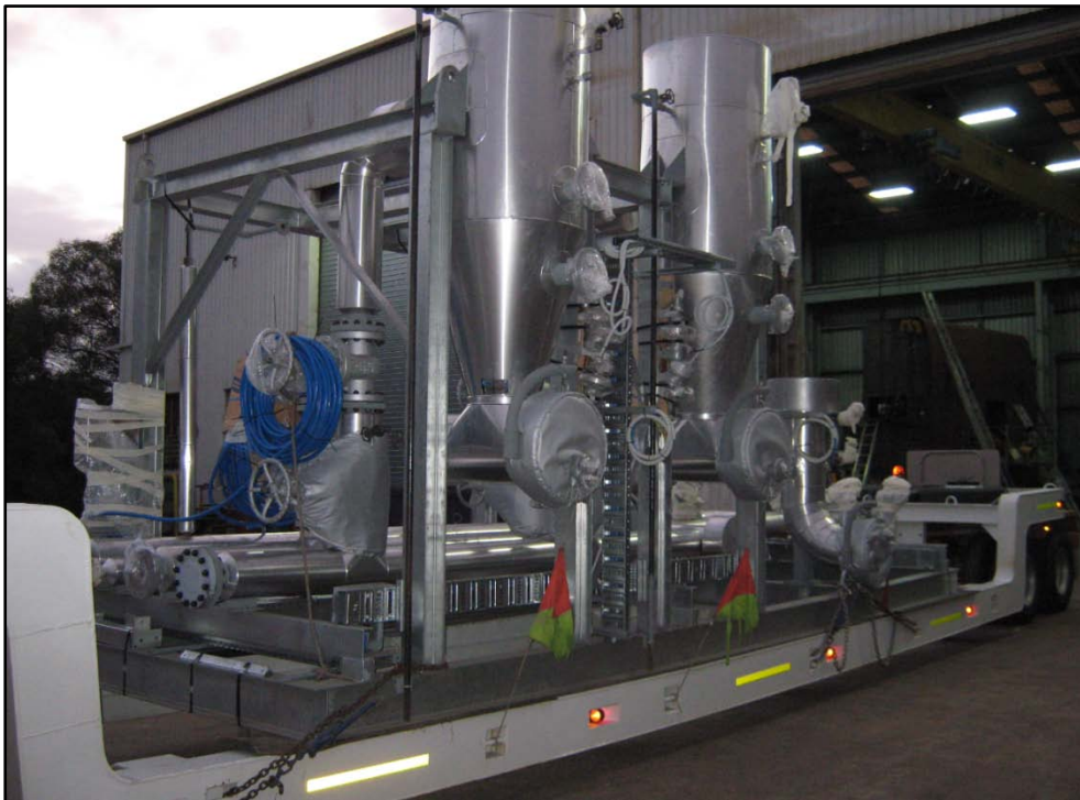
Panel 2 knock-out skid which forms part of the gas production facilities
